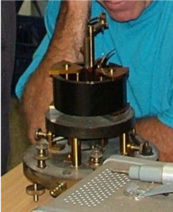
Our mirror galvanometer is missing the glass bell jar which went over the whole mechanism to keep out air currents which would have affected the reception of signals
