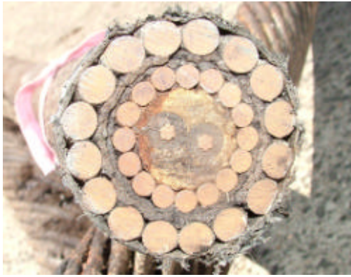
Two core submarine telegraph cable ex Darwin
