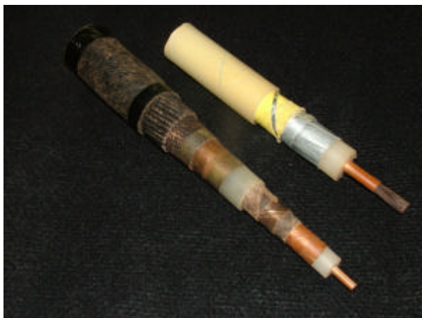
SEACOM ocean cable (top) and Madang land Cable (bottom)
